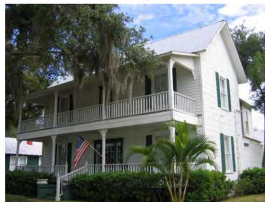
**Porch:** A structure attached to a building to shelter an entrance or to serve as a semi-enclosed space, usually roofed and generally open-sided. Differentiated from a Loggia as an “additive” element instead of a “deductive” element. (Variant: **Portico**)
